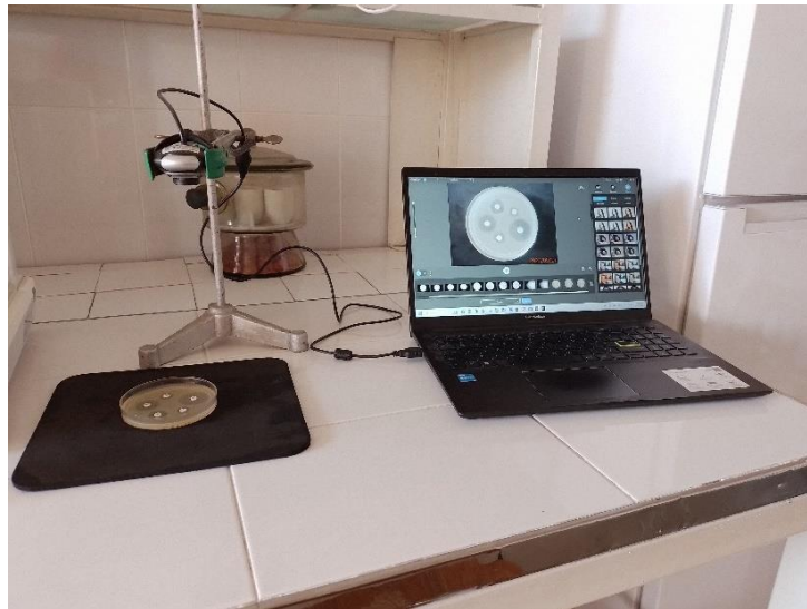
Fig. 1. The experimental device for the automatic interpretation of the antibiogram using MATLAB
